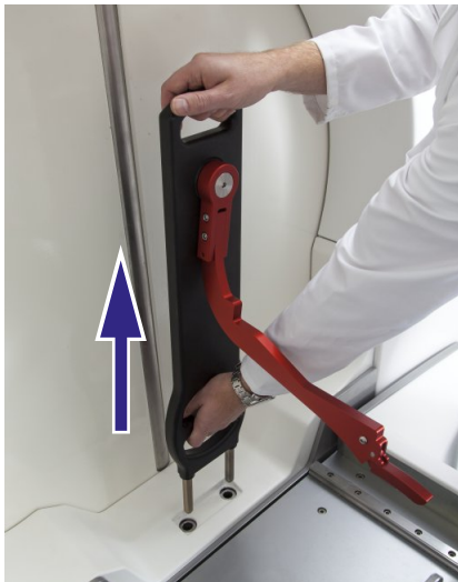
Figure 5.60 Removal of the clearance tool
