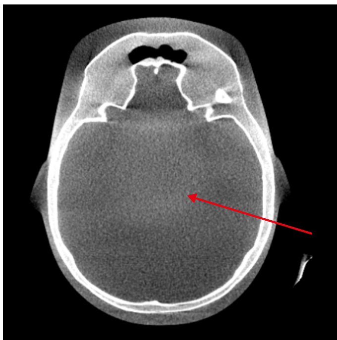
Figure 7.16 Example of non-uniformity in a uniform area of an antropomorphical phantom. There are several sources of non-uniformity for example scattered radiation, beam hardening, detector lagging and ghosting.
