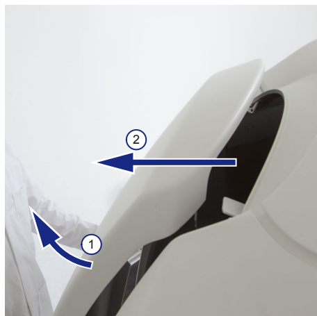
Figure 5.96 Removing the rear section of the radiation unit cover
