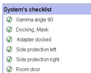
Figure 4.10 Interlock status in the System's checklist
